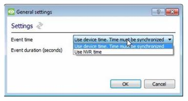
As this integration is time-critical, the event time can be set to **Use device time**, or **Use NVR time**.
