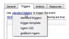
To define which device will be used to trigger the event, click on the hyperlink after "use". To set it as the Grakkom Ngaro device, click on the hyperlink, and select the device name from the dropdown menu.
